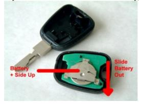
Note the position of the battery (positive side up), slide old battery out and slide in new battery.
