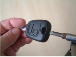
Remove key from any key rings. Using a coin or screwdriver in the slot at the rear of the key, carefully prize open the casing (some keys may also have a screw on the back of key, remove if present)
